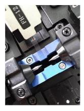
Figure 5.1 V groove cleaning I
