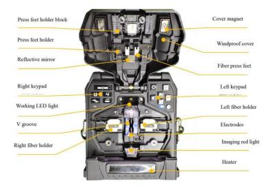
Figure 2.2 Main Structure Parts
