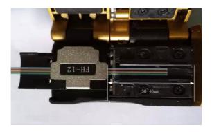
Figure 3.2 Heat stripper for ribbon fiber coating layer
