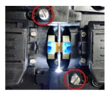
Figure 5.5-1 Remove the electrodes cover
