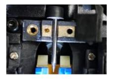
Figure 5.6-2 take out the electrodes
