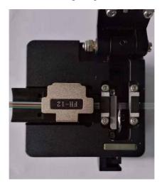
Figure 3.3 Cutting ribbon fiber
